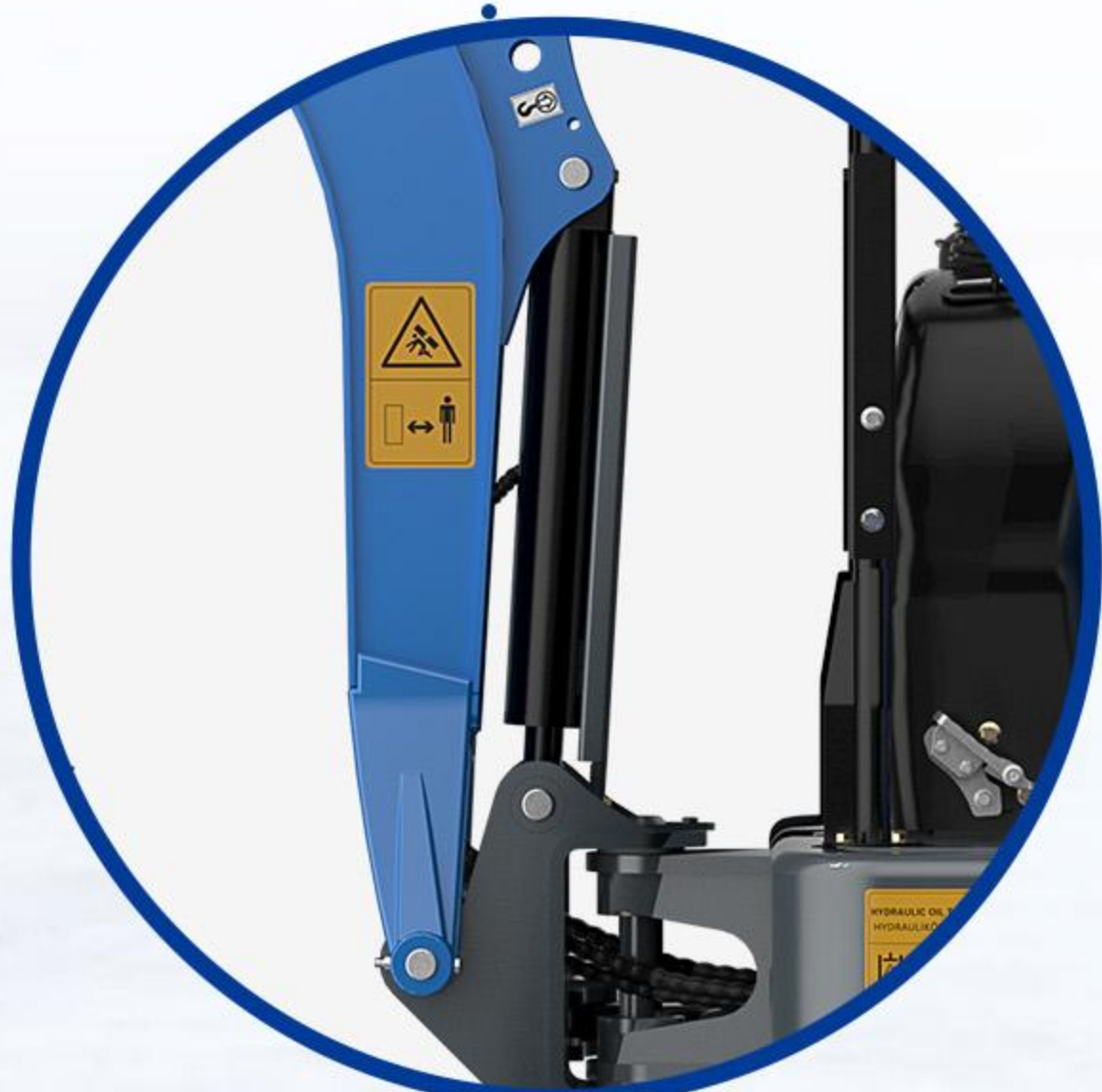
Top-mounted boom cylinder + cylinder guard plate
