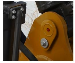
External lubrication points: The grease lubricating oil pipes are drawn out from the pin shaft and bushing, making maintenance easy.
