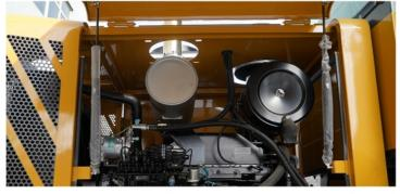
The large-opening hood can be opened upward 90°, providing a large space for maintenance; the air filter and fuel filter are centrally arranged.
