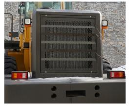
The horizontal radiator has small medium flow resistance and good heat dissipation effect.
