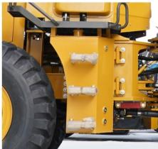
The hydraulic oil tank refueling port and torque converter oil filter are externally located for easy maintenance;
