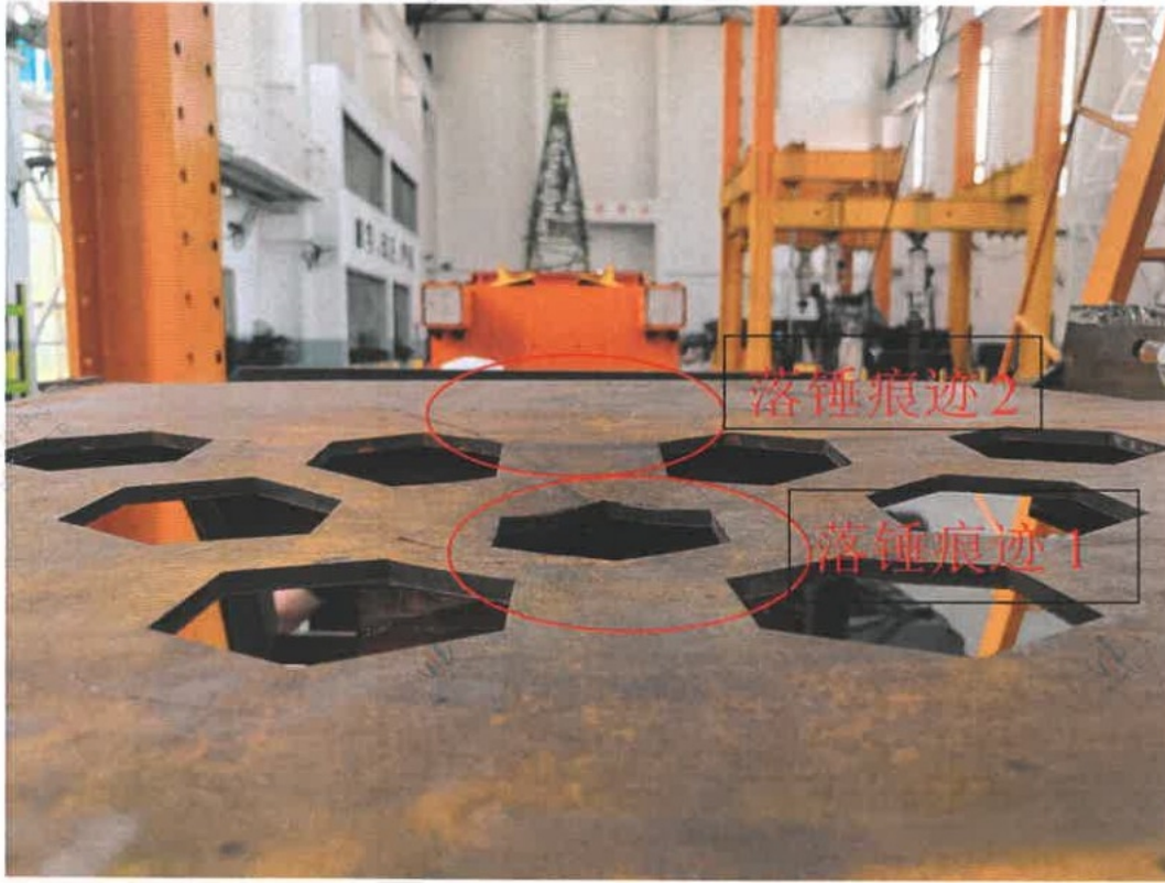
Photo-F-1 Hammer drop test
