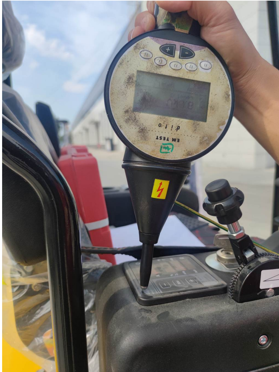
Photograph 2: Set-up for immunity test of ESD
