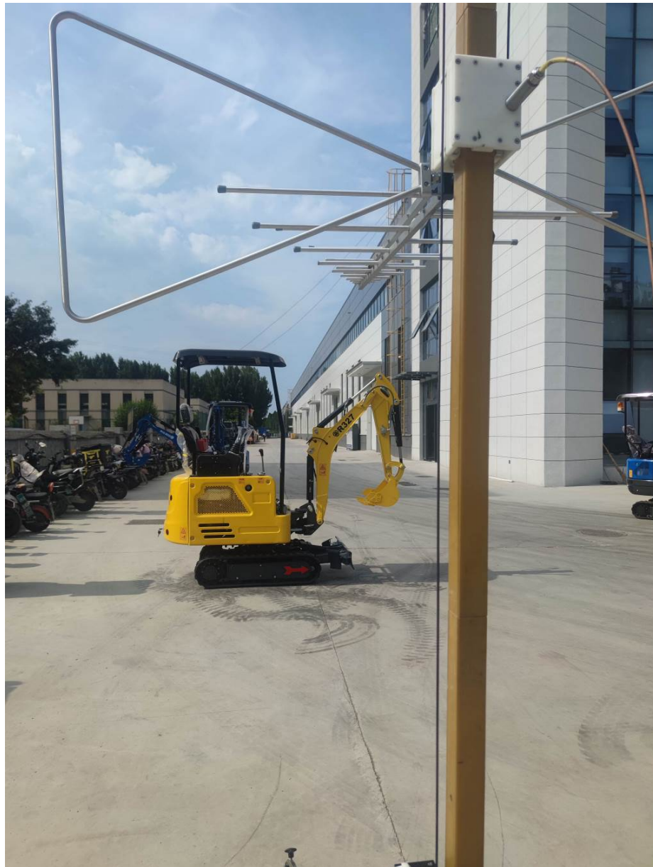
Photograph 1: Set-up for radiated electromagnetic disturbances above 30MHz
