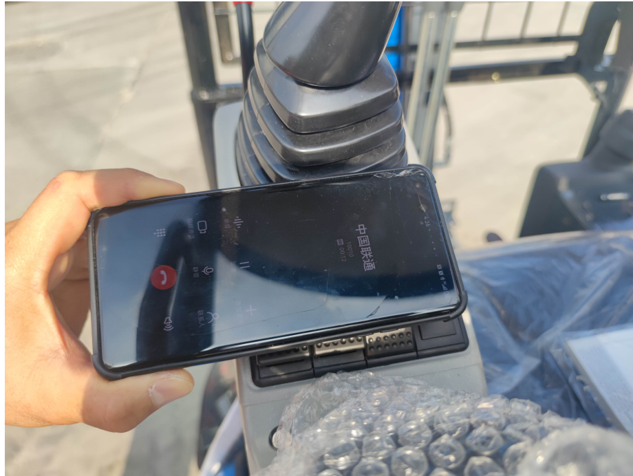
Photograph 3: Set-up for radio frequency electromagnetic field
