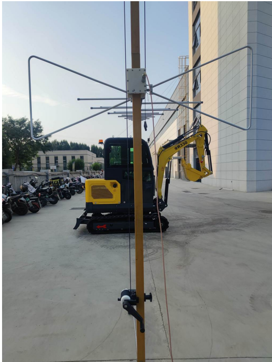
Photograph 1: Set-up for radiated electromagnetic disturbances above 30MHz
