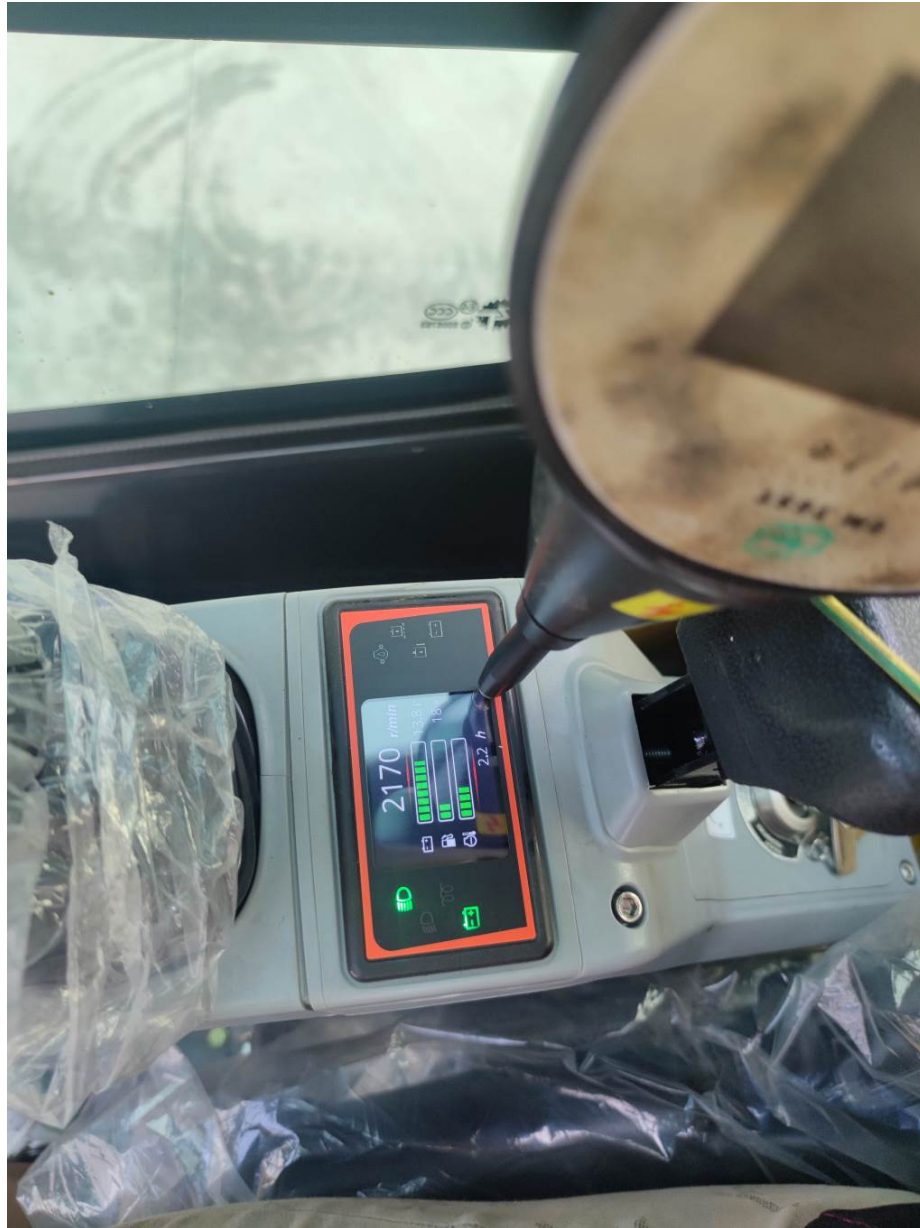
Photograph 2: Set-up for immunity test of ESD
