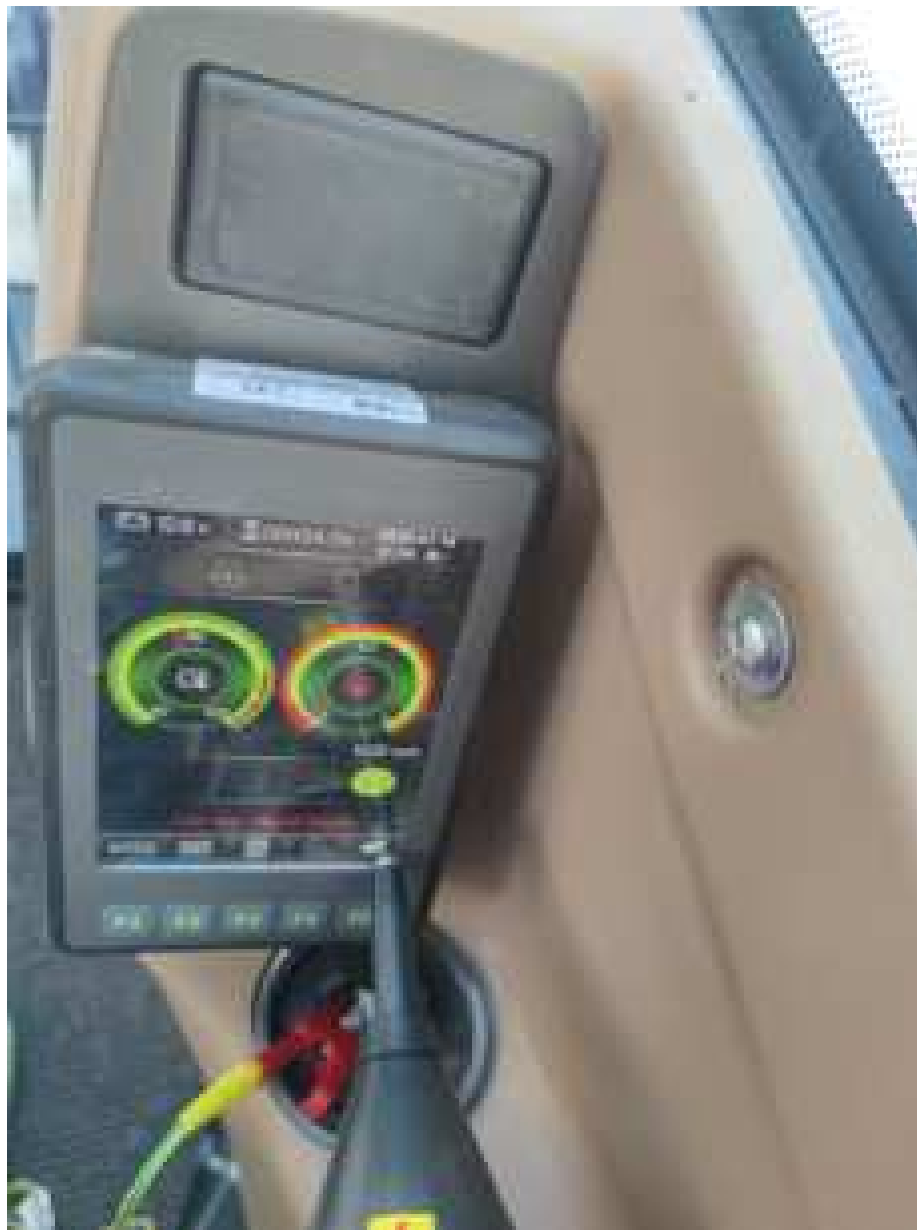
Photograph 2: Set-up for immunity test of ESD
