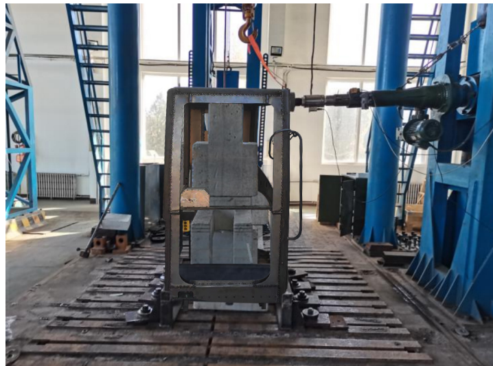
Figure. F1 Before the lateral loading test
