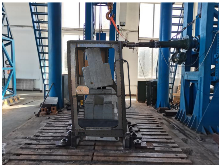
Figure. F2 After the lateral loading test
