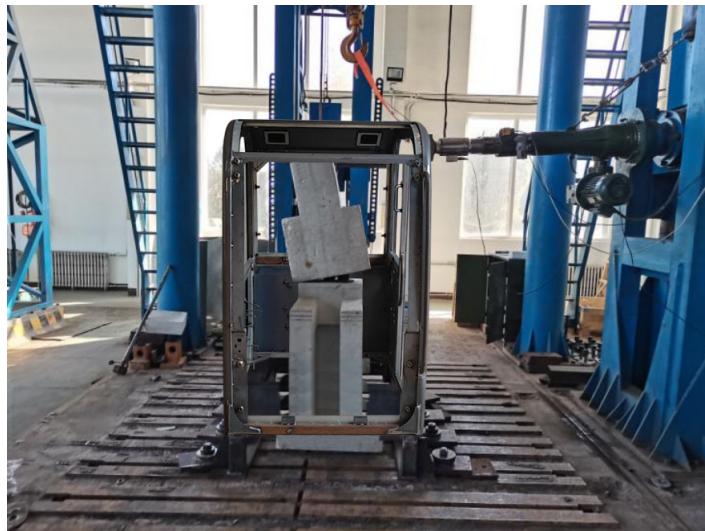
Figure. F1 Before the lateral loading test
