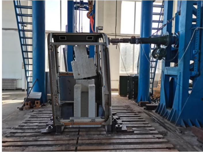
Figure. F2 After the lateral loading test
